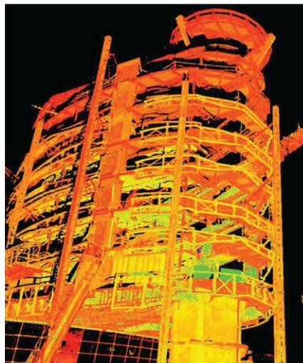
Above and left: Tronnes used the Leica ScanStation C10 laser scanner to capture accurate as-built data on the EIA Combined Office Tower.
