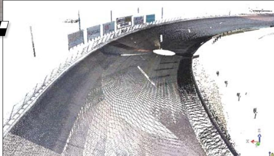
Deliverables for the project called for stripes to be located accurately. Since Darlington's stripes were nonreflective and difficult to scan, this could have meant a lot of extra total station shots. But the GX, controlled by Trimble PointScape software, took georeferenced photos that could be aligned with known points in the scanned data. “One of the cool things about the GX,” Peterson says, “was that we were able to take images from the scanner and apply them (in
